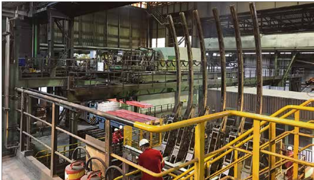
Dummy bars at the start of casting: as high as 30 m, beneath the shop ceiling.
